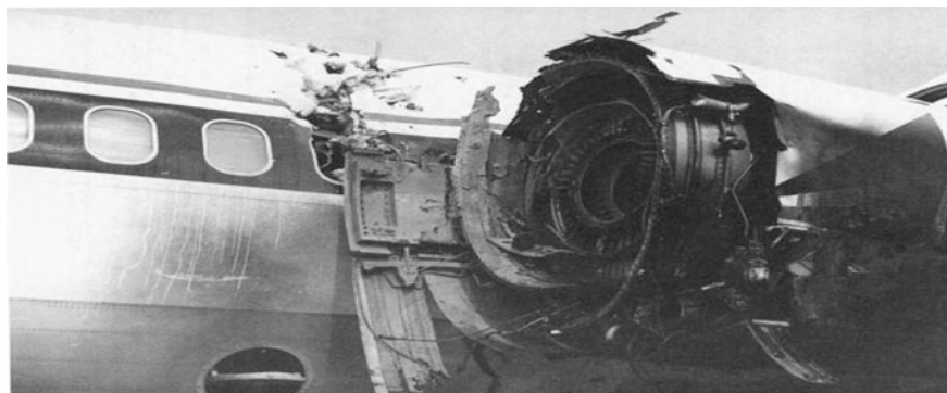
Fig. 1 Engine of Delta Air Lines Flight 1288 after it experienced catastrophic uncontained compressor rotor failure in 1996 (NTSB Report of Delta 1288, January 13, 1998)
