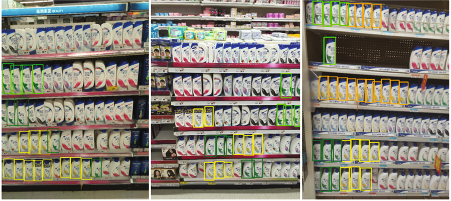
Fig. 8. Selected examples of object detection results on the shampoo data set using our system, illustrating that our system can successfully detect the objects of interest.
