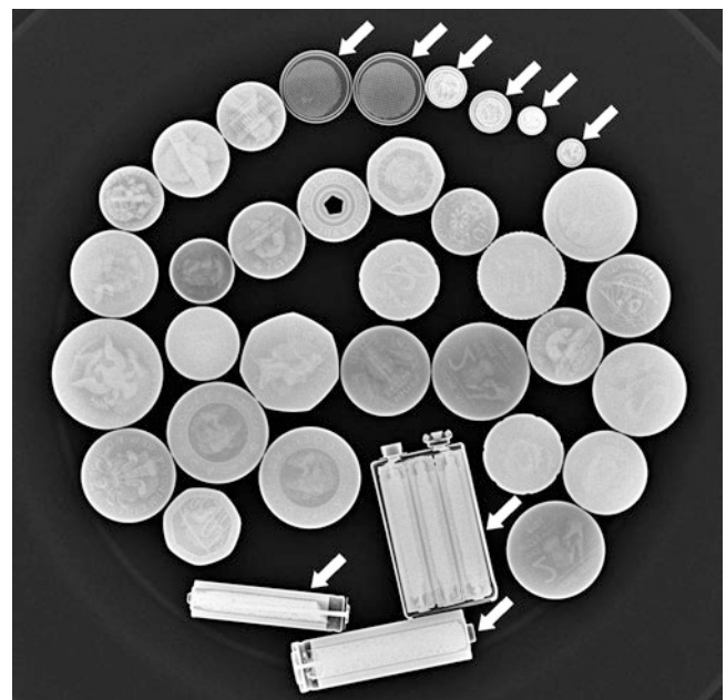
Fig. 26.12 Radiography of coins and batteries. Beveled edge appearance differentiates disk batteries coins. Batteries (disk, AA, A and 9-volt batteries) are identified with arrows in the radiograph
