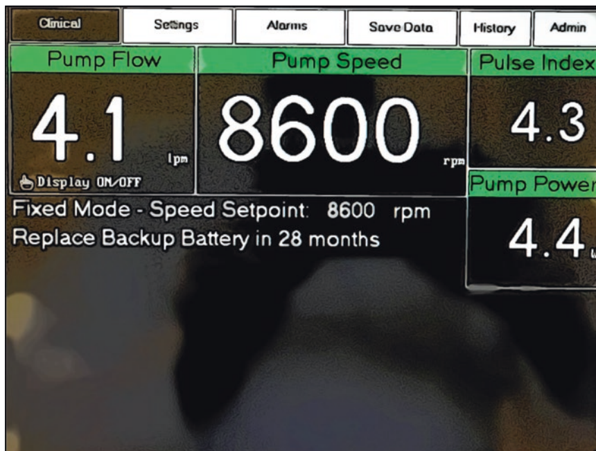
Fig. 10.7 HeartMate II display panel. The pump speed, pump power, pulsatility index, and pump power are displayed
