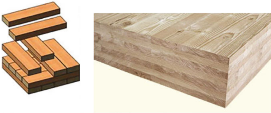
Fig. 5.14 Cross-laminated timber manufacture
