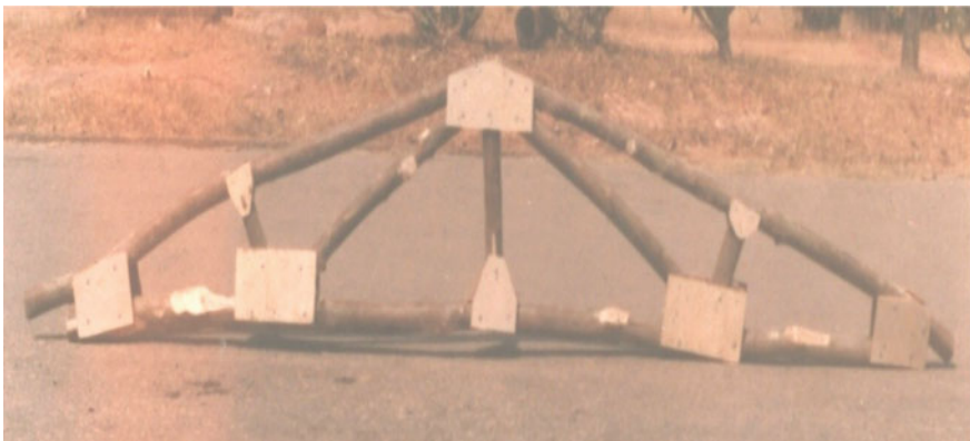
Fig. 12.3 Side view of the truss fabricated with branches of guava tree. Source Lucas et al. (2006)
