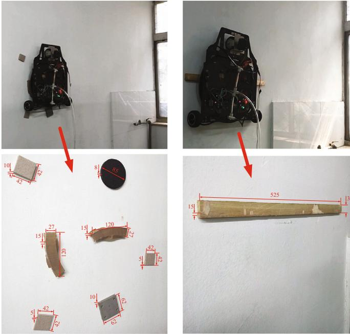
Fig. 16. Experiment on a smooth wall with raised obstacles
