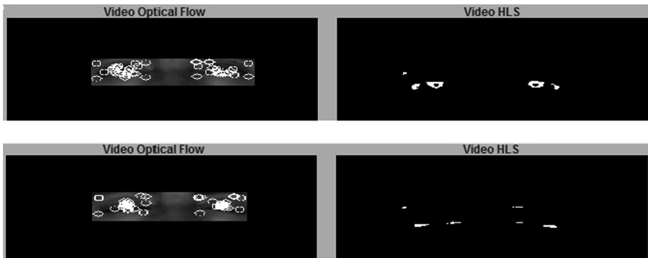
Fig. 5. Top: TER with open eyes converted to the HLS color space. Bottom: TER with closed eyes converted to the HLS color space
