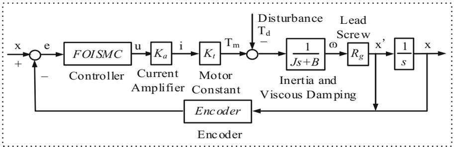
Fig. 2. Fractional-order sliding mode control scheme
