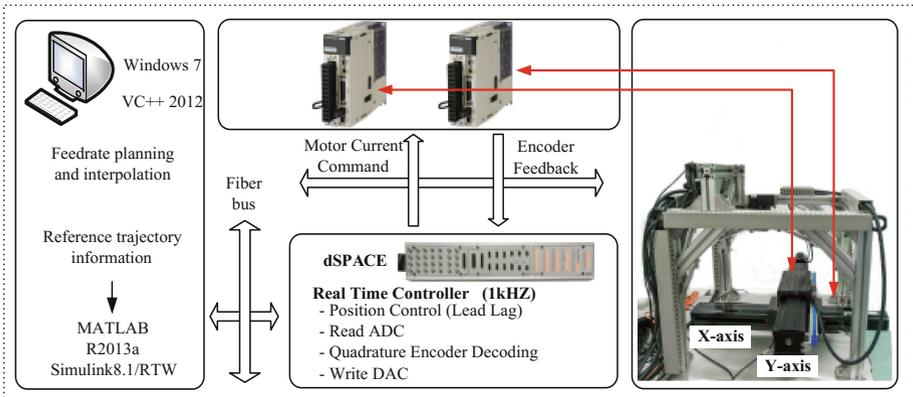
**Fig. 3.** Experimental platform of the biaxial table
