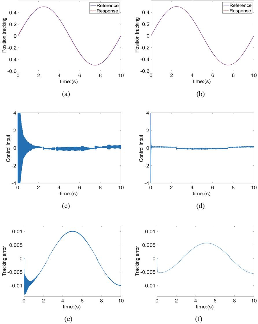
**Fig. 4.** Sinusoidal responses. (a), (c) and (e) Traditional SMC. (b), (d) and (f) Proposed FOISM C.
