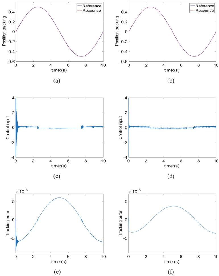
**Fig. 6.** Sinusoidal responses. (a), (c) and (e) Traditional SMC. (b), (d) and (f) Proposed FOISM.
