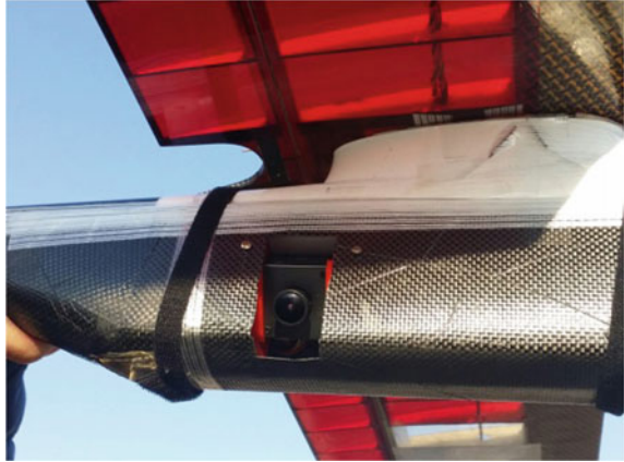
Fig. 11 Fixed-camera on the test bed aircraft looking out to the side
