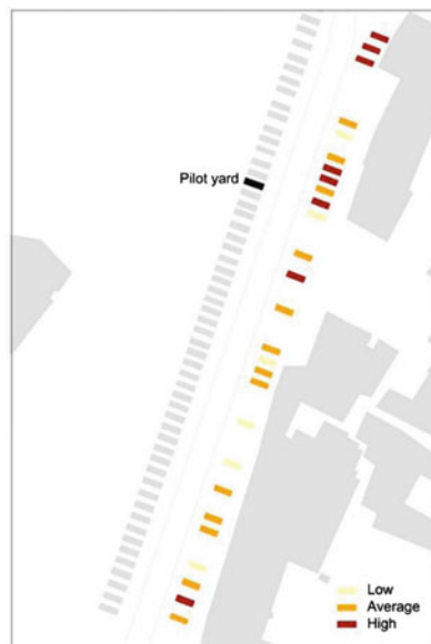
Fig. 13 Severity levels of decay phenomena. Examples for “alteration of the visual aspect and color” and “loss of mechanical strength”
