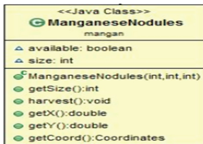
Fig. 3. Visual class diagram ManganeseNodule .
