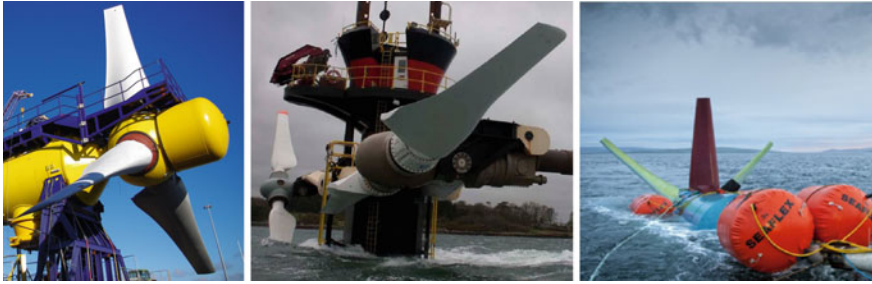
Fig. 1 Various tidal energy blades in situ, manufactured by AEL/Airborne
