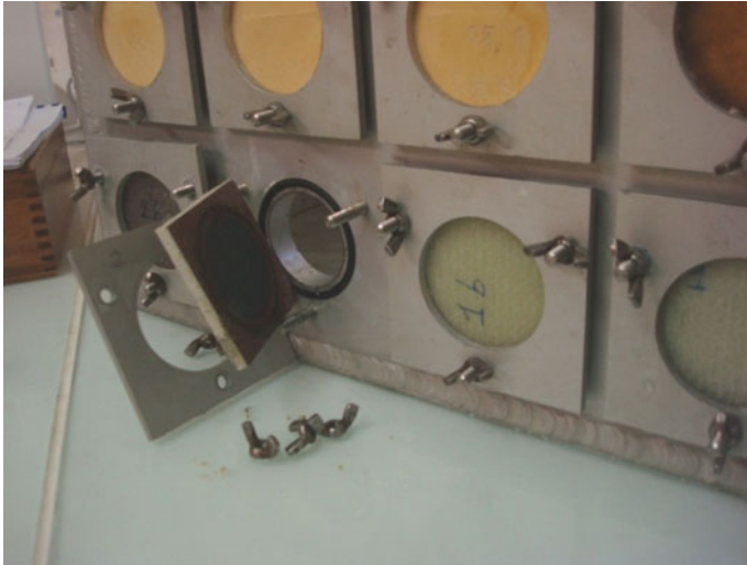
Fig. 7 Ageing setup for one-sided exposure of 70 \times 70 \text{ mm}^2 samples to seawater
