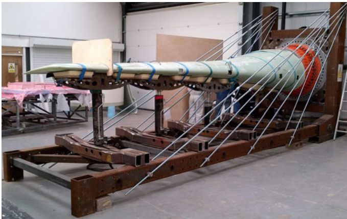
Fig. 5 Tidal energy blade static test at AEL
