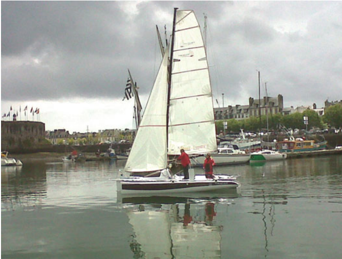
Fig. 9 Gwalaz all-flax reinforcement trimaran
