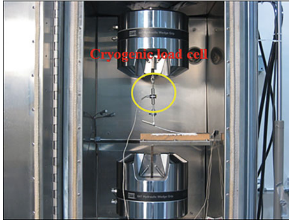
Fig. 13 DCB specimen testing setup for interface delamination studies that shows cryogenic load cell
