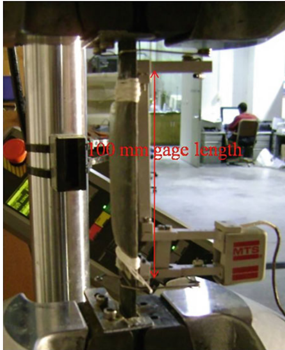
Fig. 10 One-sided seawater confinement/exposure for [\pm 45]_{2S} specimen and tension–tension ( R = 0.2 , 1 Hz) cyclic fatigue setup, 100 mm gage length corresponds to distance between knife edges of extensometer on the gage section
