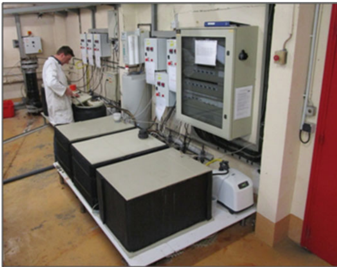
Fig. 2 Natural seawater ageing tanks maintained at different temperatures and continuously renewed
