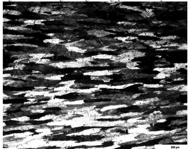
Figure 5: Mid thickness grains, low casting speed, 8079 alloy.
