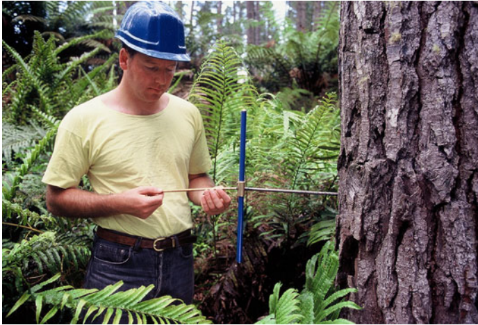
Fig. 6.11 Collection and preliminary field evaluation of increment core which can be used for determination of several wood properties in addition to density
