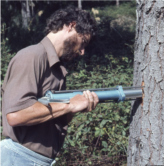
Fig. 6.10 Field operation of penetrometer used to measure wood density on standing radiata pine. This gave less accurate determinations than using increment cores, but that was offset by allowing determinations on more trees for given time and budget
