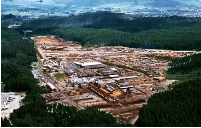
Fig. 3.2 Aerial photo of Waipa Sawmill near Rotorua, New Zealand, built by the State Forest Service to pioneer large-scale processing of exotic species. Opened in 1939, it became the largest sawmill in the Southern Hemisphere. Note the very large yard for drying sawtimber in the open
