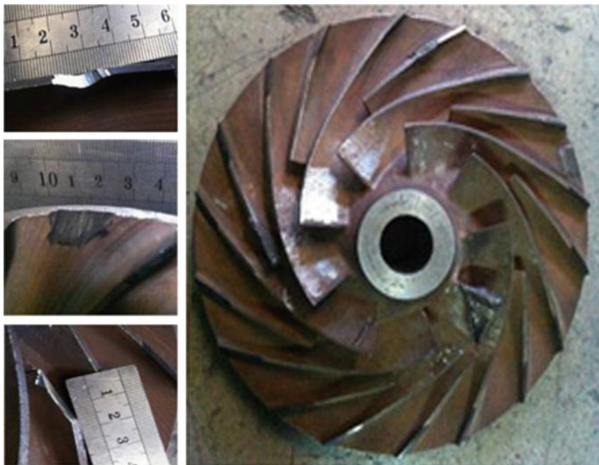
Fig. 7.12 Failed open impeller [34]
