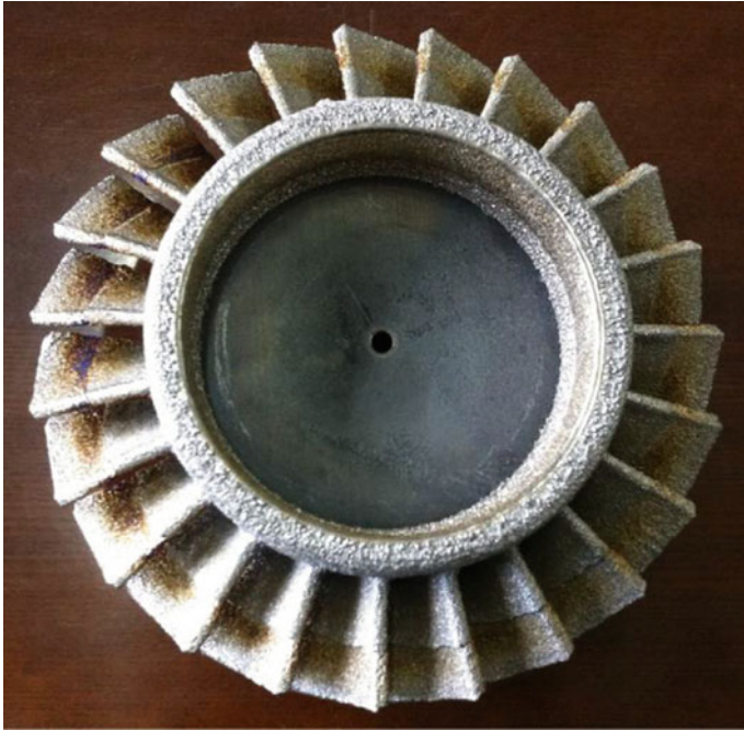
Fig. 3.11 Direct laser deposited TC11/Ti2AlNb dual alloy blisk [29]
