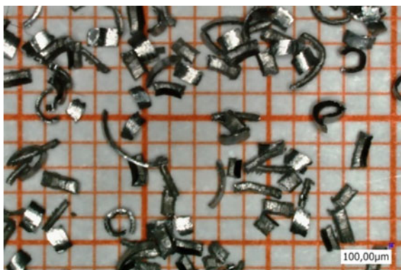
Fig. 12 Chips dimensions with MWF supply of 1.91 L/min (40 bar)
