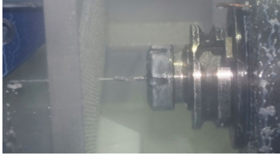
Fig. 17 MWF supply is insufficient for through holes
