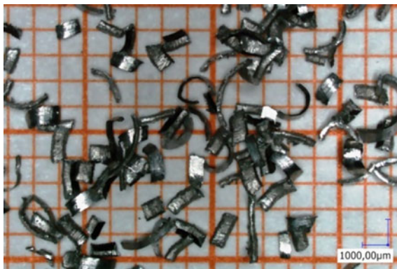
Fig. 11 Chips dimensions with MWF supply of 1.19 L/min (20 bar)
