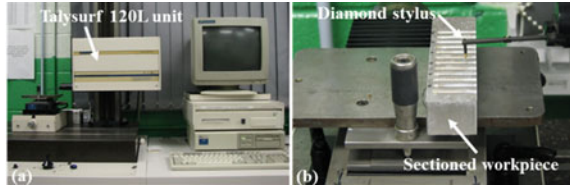
Fig. 4 Hole surface roughness evaluation. a Form Talysurf 120L unit and b measurement setup
