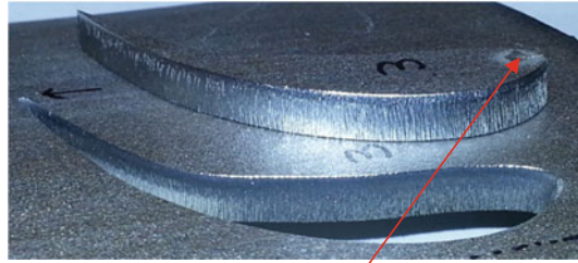
Small clean pierce without any spatter
