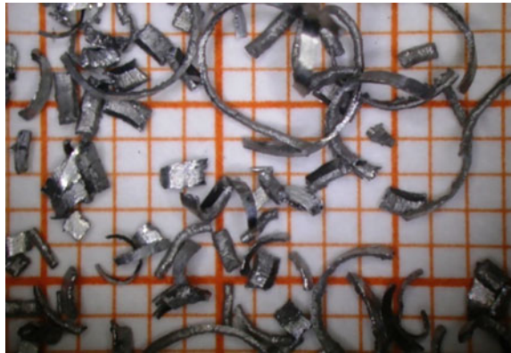
Fig. 10 Chips dimensions with no MWF supply
