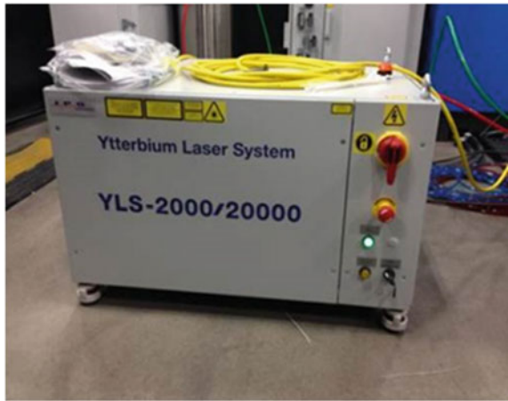
Fig. 7 IPG 20 kW QCW fiber laser; 20 kW peak power; 2 kW average power; 200 J pulse energy
