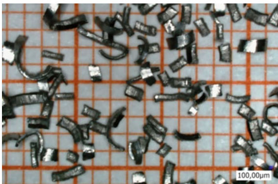
Fig. 13 Chips dimensions with MWF supply of 2.65 L/min (80 bar)
