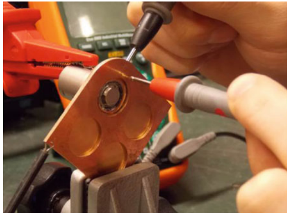
Fig. 18 Measurement of the electrical resistance
