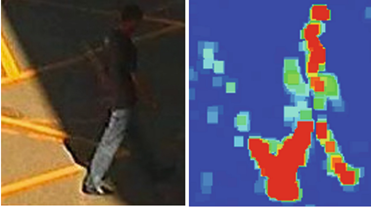
Fig. 6. Reliability map using naive background subtraction. Left image: current image, right image: reliability map from naive background subtraction.
