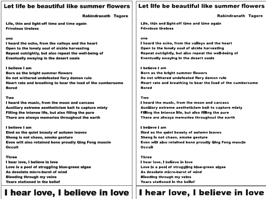
Fig. 9. Vectorization of a typed document page. Left: the input document, right: the vectorized result. The input image suffers from aliasing when the page is scaled and our result can keep the shape of each character well.
