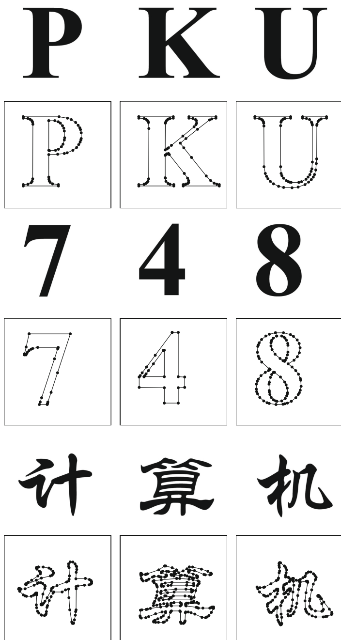
Fig. 5. Vectorization results of different characters. The first, third and fifth rows are input raster images(English, Digit and Chinese characters respectively), the second, fourth and sixth rows are corresponding vectorization results with contour represented by line segments.
