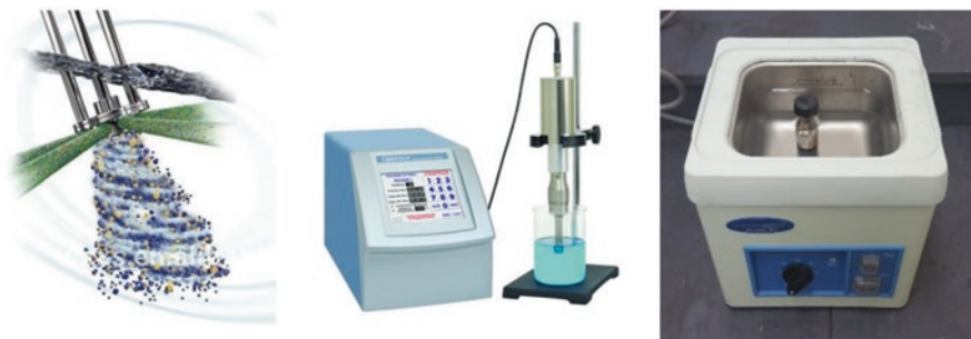
Fig. 1.11 Left to right: Shear mixer ( http://www.silverson.com/us/products/batch-mixers/ ), tip (horn) sonicator (photo of Q500 Sonicator from Qsonica), and bath sonicator
