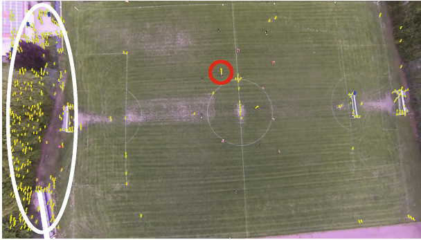
Fig. 2. Video image from the Soccer sequence with inliers and their trajectories (yellow lines) after KLT & RANSAC. The inliers are highly clustered at 3D structures (trees/houses) on the left (white ellipse). Moreover, a correspondence located at a player was erroneously considered as inlier (red circle). (Color figure online)
