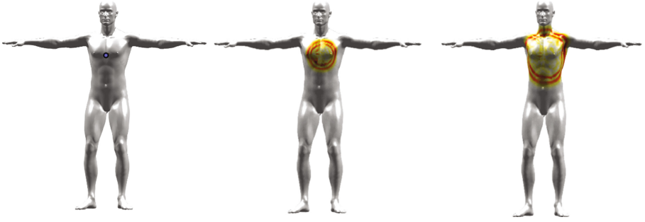
Fig. 2. The dynamics described by the wave equation on a triangular meshed surface. In this case, the solution was modelled with the BT scheme. The initial point displacement u(p, 0) = \delta_{blue}(p) takes place at the blue point on the man’s chest. The time evolution of |u| is shown from left to the right. (Color figure online)
