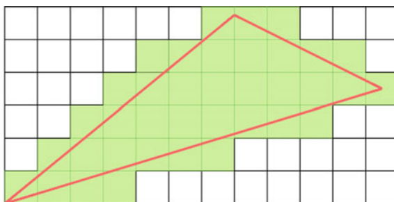
Fig. 5 The choice of important cells from the point of view of the mission ( green ) on the basis of the area of the mission (limited red lines)
