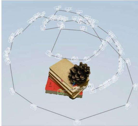
Fig. 20 3D model reconstructed in 123D Catch software using a series of 67 images
