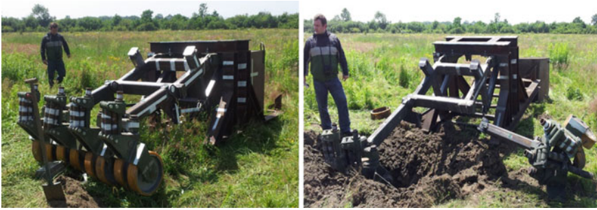
Fig. 23 Anti-mine vehicle after destructive testing
