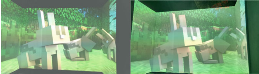
Fig. 8 (Left) The calibration result for p = 1 correction factor G (Right) calibration result for p = 1.9 correction factor G
