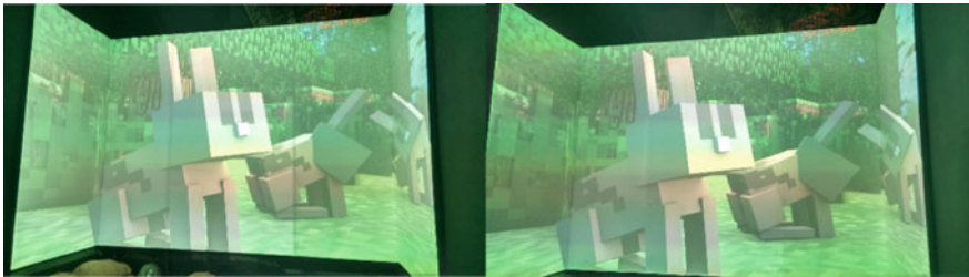
Fig. 7 (Left) The calibration result for p = 1.9 without correction coefficient G , (Right) calibration result for p = 1.9 , taking into account the coefficient G
