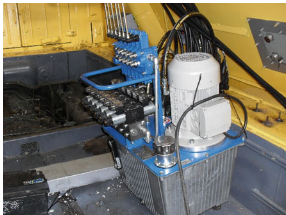
Fig. 7 The photography of hydraulic pump. The equipment was installed inside
