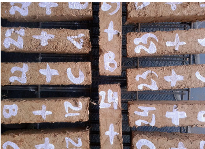
Fig. 7 Lime stabilized hemp-clay concrete test specimens
