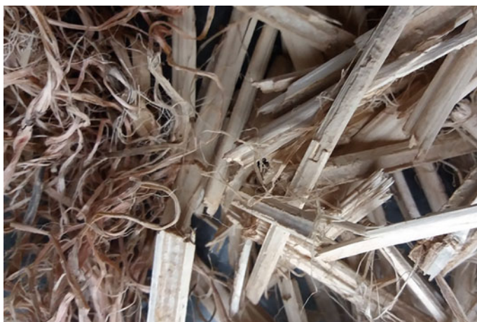
Fig. 5 Spanish hemp core and fiber after 14 days of submersion in water and drying
