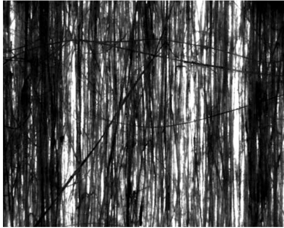
Fig. 3 Example of unidirectional ply of flax [19] (without matrix). Some of the fibres (elementary fibre or bundle of fibres) are not aligned in the longitudinal direction, but such misalignment is minor
