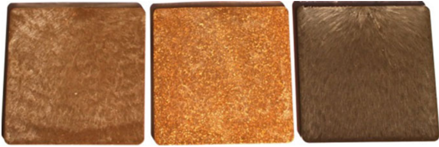
Fig. 1 Injection moulded PLA-fibre composites with hemp dust ( left ), shives ( middle ) and hemp fibre ( right )
