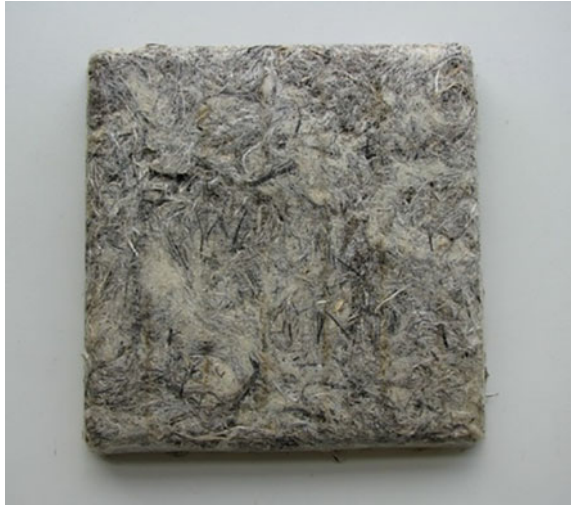
Fig. 1 Bio-composites specimen of wool and hemp board (10 × 10 cm)
