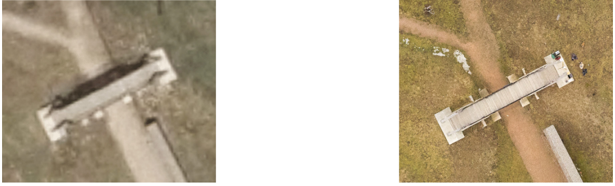
Fig. 3. A detail of the orthophoto from the CUZK [5] (left) and the orthophoto produced by the UAV photogrammetry (right).
