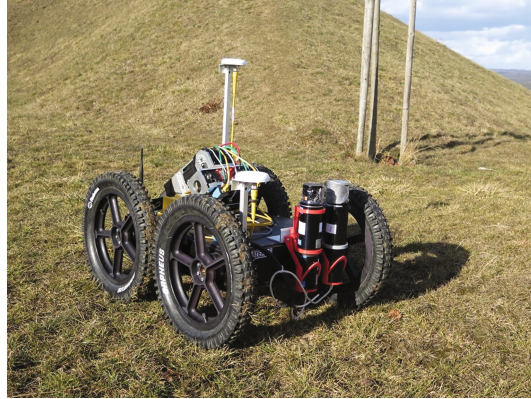
Fig. 8. Robot carrying equipment for gamma radiation measurement.
