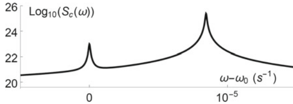
Fig. 3 The power spectral density of the output optical field phase quadrature predicted by the Schrödinger-Newton equation for the Levitating Mirror
