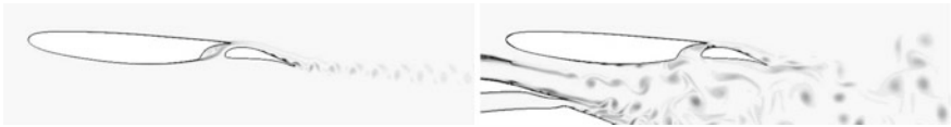
Fig. 7 2D wing without (left) and with nozzle (right). Contour levels of the vorticity magnitude |\omega_z| . The grey scale ranges from 0 up to the level of 50U_s/D_s , from white to black
