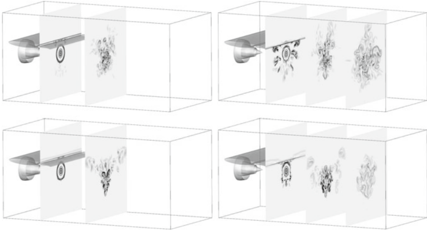
Fig. 11 3D jet-wing-flap configuration with U_\infty = 0 (top) and U_\infty = 0.467U_s (bottom): Snapshots of vorticity magnitude in the (y, z) -planes at x = 1.5D_s and 3.75D_s (left); at x = 2D_s, 4D_s and 6D_s (right). The grey scale ranges from 0 up to the level of 15U_s/D_s , from white to black
