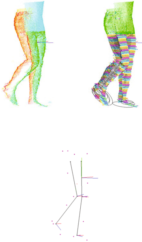
Fig. 11. The algorithm of virtual markers calculation: initial data (left), segmentation by slicing (middle) and final bones and markers (right)
