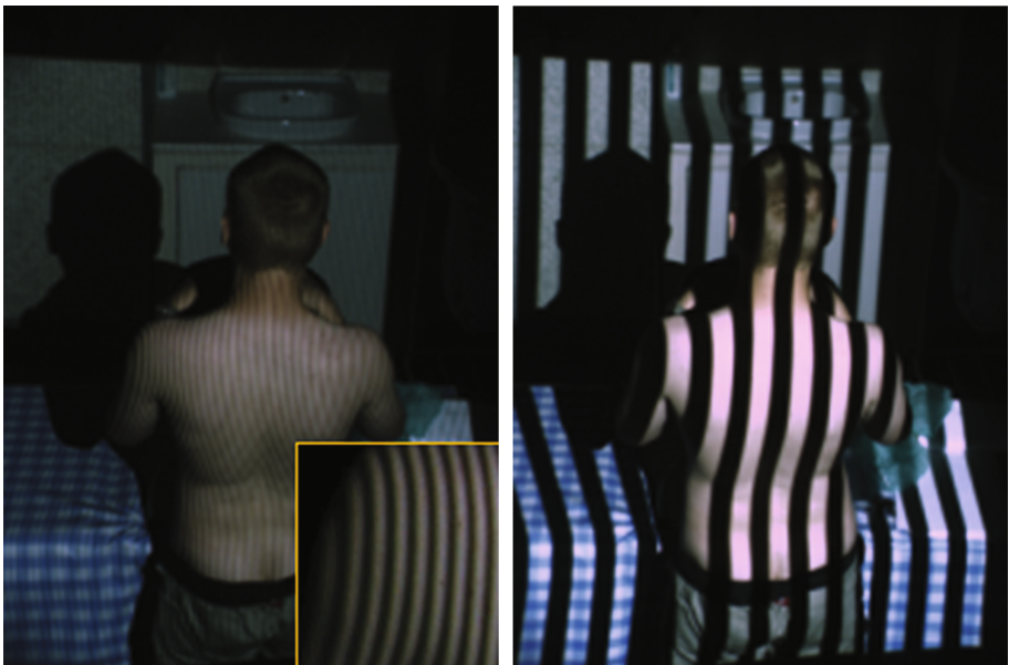
Fig. 1. Exemplary images from measurement sequence: sinusoidal pattern (left) and Gray code (right)
