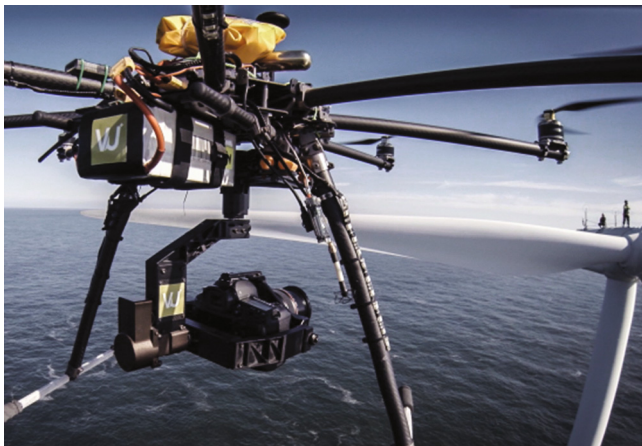
Fig. 8. Inspection of WTGs by a specialized drone [10]
