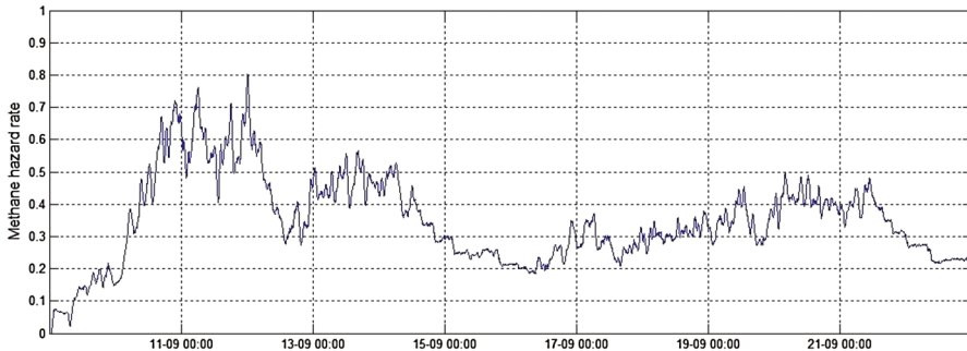
Fig. 2. Methane hazard rate during trials carried out at the working face area
