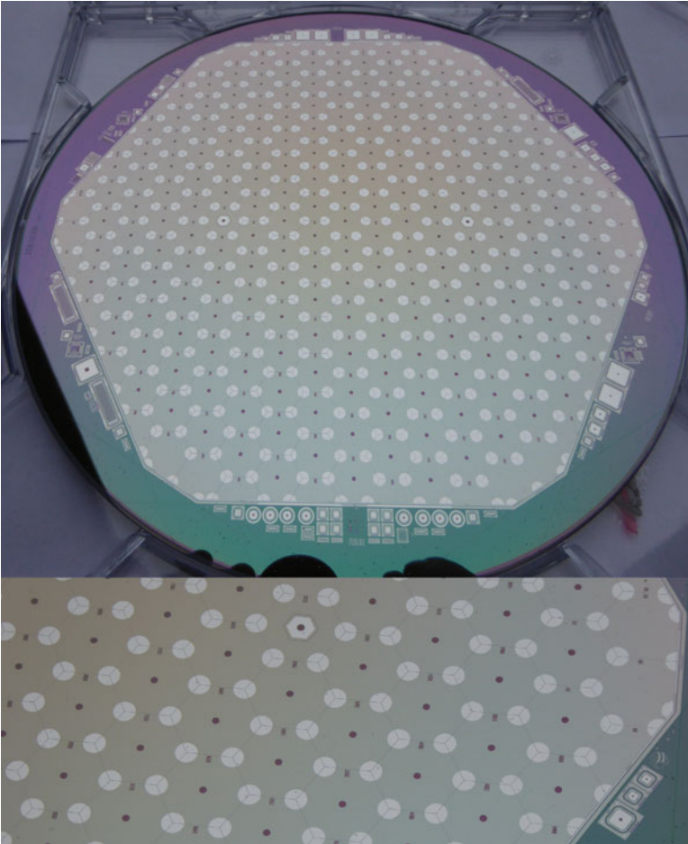
Fig. 7.27 Photo of an 8 in. HGC prototype wafer scaled down by a factor 2. The hexagonal structure optimizes the use of the wafer surface and can finally be tiled to cover a flat surface with minimal inactive areas. Below, a zoomed view of the right wafer corner is shown. All readout cells are hexagonal. The circles at the cell corners are openings in the passivation to allow wire-bonding. Two wafer cells have an extra smaller pad in the centre with smaller capacitance (thus lower noise) allowing for more precise calibration of MIP signals
