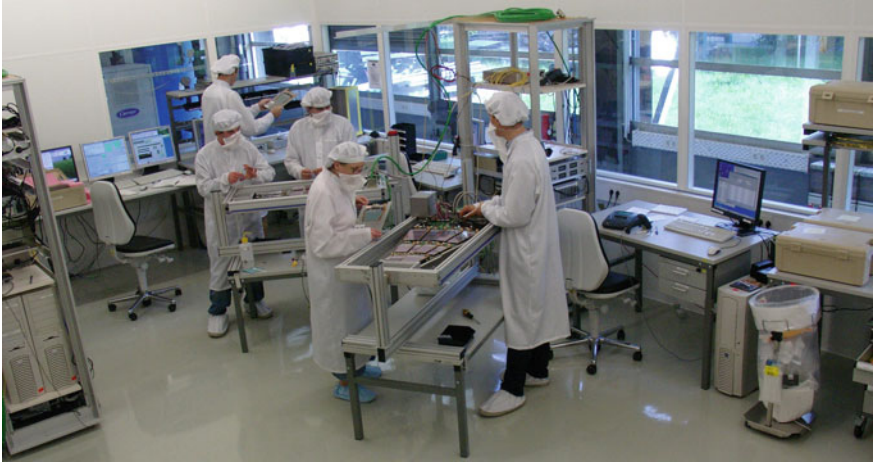
Fig. 6.37 Petal integration in Karlsruhe. Three technicians plus two physicists were assembling two petals simultaneously. The petals were mounted on so-called petal grills which enable easy turnaround and thus access to both sides. After assembly, petals were long-term tested in fridges with additional active petal cooling
