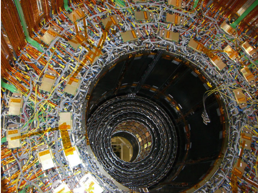
Fig. 6.18 TIB inserted in TOB, a rare view. The four layers of the tracker inner barrel are visible inside the tracker outer barrel. The TOB layers 5 – 10 are completely hidden by the necessary cabling. This is a rare view during the time of construction
