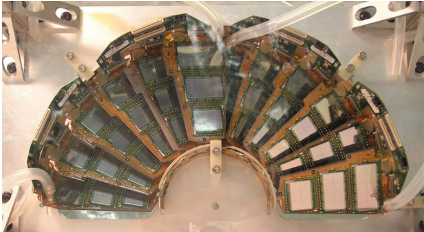
Fig. 6.4 One of the forward half-disks. Please note the turbine configuration emphasising the Lorentz angle spread. To achieve a wedge geometry seven different sensor geometries, assembled on so-called panels, have been produced. Eight half-disks, forming 4 full disks, 2 at each end, finally surround the beam pipe [Courtesy of CMS/CERN/FNAL]
