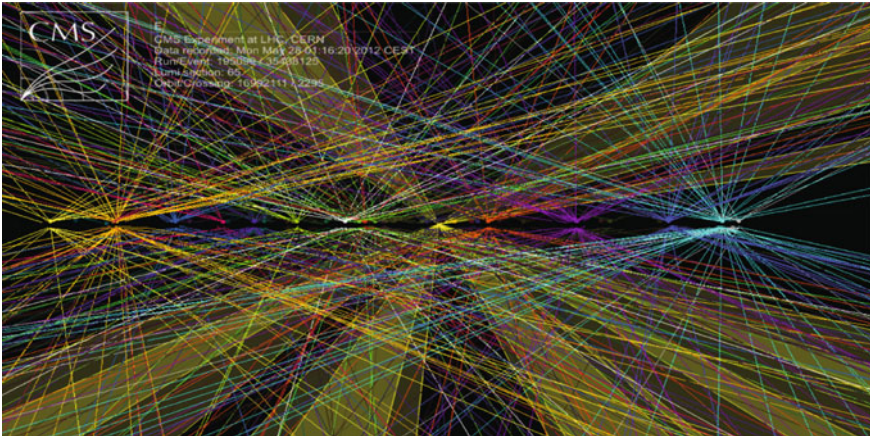
Fig. 6.49 The situation at high pile-up of about \text{PU}=45 with about 1500 tracks cross the CMS tracker every 25 ns. The spacing between individual vertices is about 1 - 2 \text{ mm} [Courtesy of CMS/CERN]
