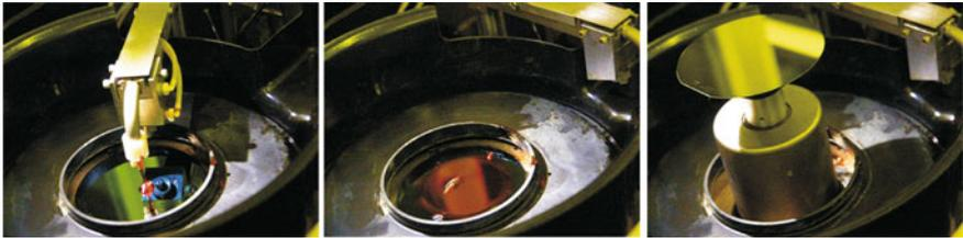
**Fig. 1.55** Photoresist is roughly spilled in the middle of the wafer, centrifugal forces, during fast rotation, homogeneously distributes the resist on the wafer. Courtesy of ITE Warsaw [347]
