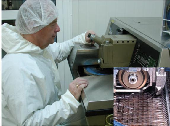
**Fig. 1.66** A CMS sensor cut from its wafer. The blue foil, the wafer rests on, was not cut
