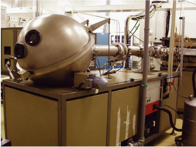
**Fig. 1.58** The picture shows an ion implanter. Ions are accelerated and guided onto the target inside the sphere, where several wafers are rotated and homogeneously hit. The ions do not penetrate through the masking layer ( $\text{SiO}_2$  or photoresist), therefore well-defined patterns, e.g. strips/pixel can be implemented on the wafer. Courtesy of ITE Warsaw [208, 347]
