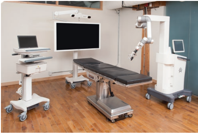
Fig. 14.1 Robotic scope holder with automatic stereotactic positioning based on the position of the access port (Courtesy of Synaptive Medical, Toronto, ON, Canada)
