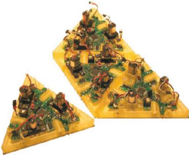
Fig. 2. Four programmable parts partially assembled into a triangle
