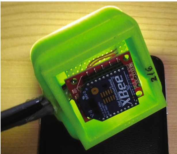
Fig. 5. “The sensor” setup – the room transmission node
