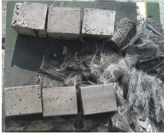
Fig. 9. Samples after 600 °C heat
