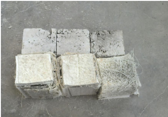
Fig. 11. Samples after 800 °C heat
