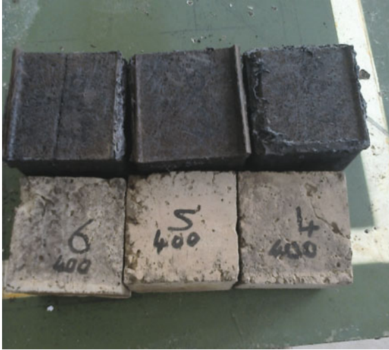
Fig. 8. Samples after 400 °C heat
