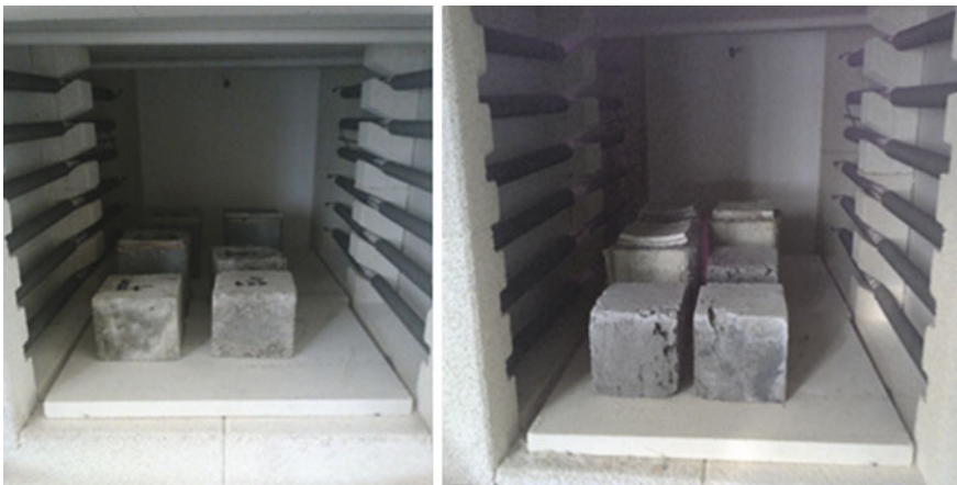
Fig. 3. Samples exposed to high temperature in furnace
