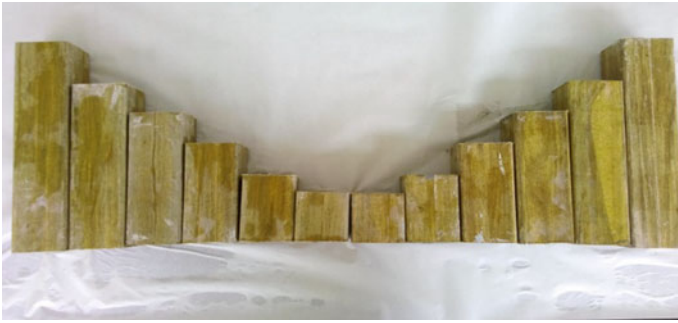
Fig. 6. Buckling test specimens
