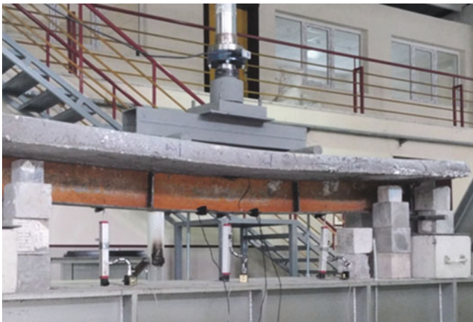
Fig. 10. Deformed shape of the un-strengthened sample
