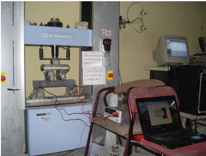
Fig. 5. Four-point flexural test together with DC-4probe electrical test
