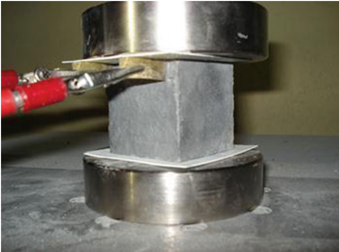
Fig. 3. Closer view of specimen taken during testing under uniaxial compression test
