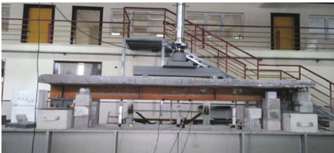
Fig. 7. Steel-concrete composite beam test set-up
