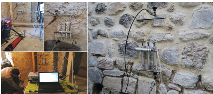
Fig. 2. Flat-jack test conducted by Kuran and Dabanlı
