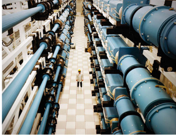
Fig. 3 The 100 kJ, 10-beam, IR, Green , or UV Nova Laser 1985
