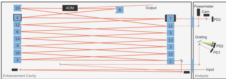
Fig. 1 Schematic of the EC. The 30-m-long EC consists of one input-coupling mirror (1, R = 99\% ) and 15 highly reflective (HR) mirrors (2–16). Two of the HR mirrors are curved (4, 12) in order to form a stable resonator (see Fig. 2a). The mirrors 8 and 9, which are plane for the steady-state experiment, are replaced by curved ones once the AOM is inserted for the non-steady-state experiment (see Fig. 2a). The beams transmitted through mirrors 7 and 11 are sent to diagnostics such as a camera (Cam) and photodiodes (PD). The photodiode behind the grating is used for the Pound–Drever–Hall stabilization scheme [29]
