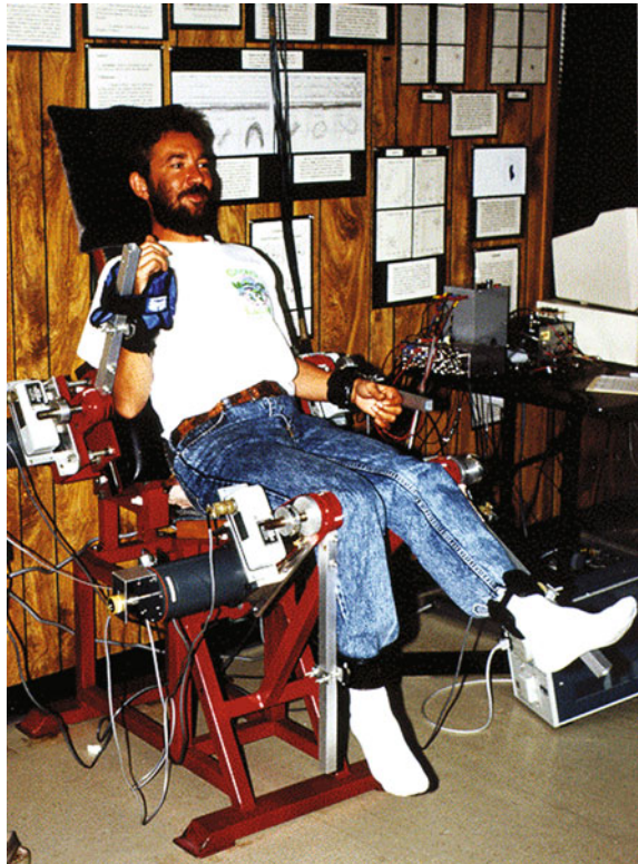
Fig. 3 A subject in the MAC (Multi-Articulation Coordination). This device allows for perturbations of the movements by applying a brake for a short moment and for varying the degree of symmetry breaking by attaching weights to either the wrist or ankle. As the legs naturally have a smaller eigenfrequency than the arms, the degree of symmetry breaking can either be further increased or reduced with loads at the ankles or wrists, respectively
