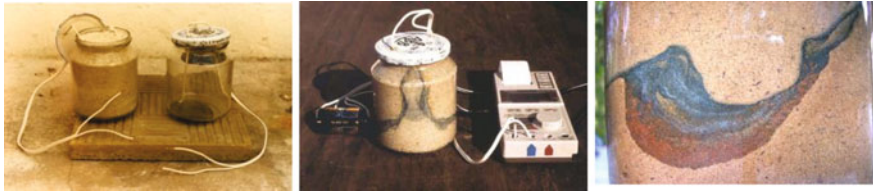
Fig. 4 (Left) Glasses with electrodes in place and already filled with moist sand, (Center) Visible effect of electric fields applied by a common battery, (Right) Development of colored redox horizon caused by electric energy input. Photographs K.-H. Jacob
