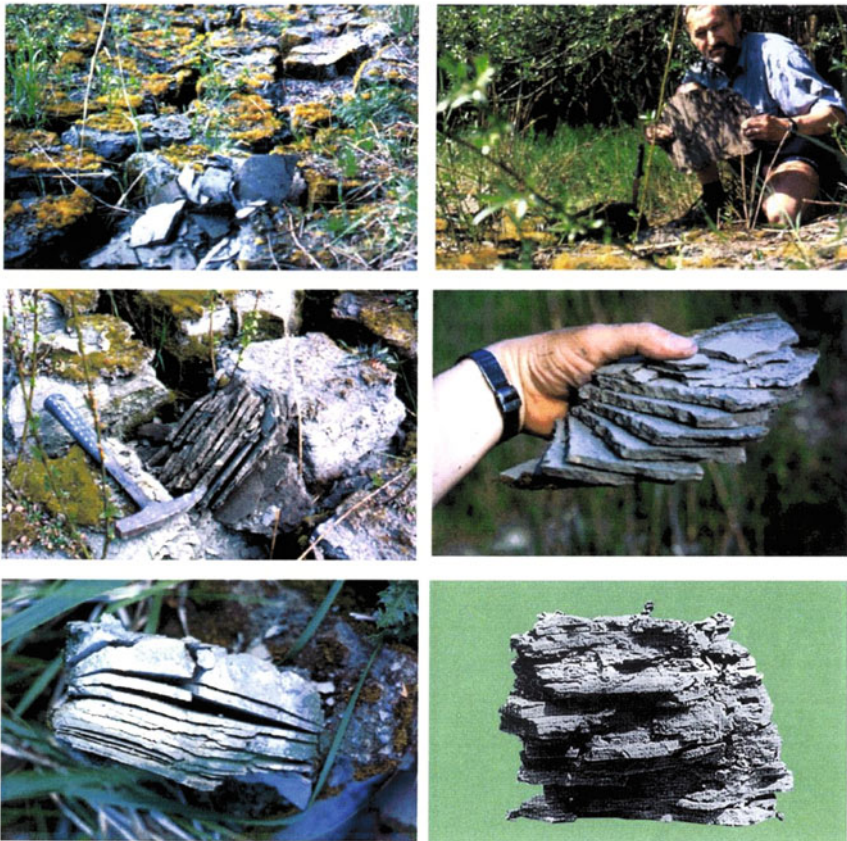
Fig. 12 The first 5 pictures were taken at a landfill only six years after the sludge had been filled in that place and stayed undisturbed. The structure shows remarkable similarity to banded “metamorphic rocks”. Striking is not only the rhythmic banding, but also the cleavage, which is characteristic for schistose rocks. The picture in the bottom left corner shows a special type of soil: the banded pararendzina (Rid [32]). Structures such as these occur relatively often in nature and could be explained by means of self-organization (Radebold [33]). Photographs K.-H. Jacob
