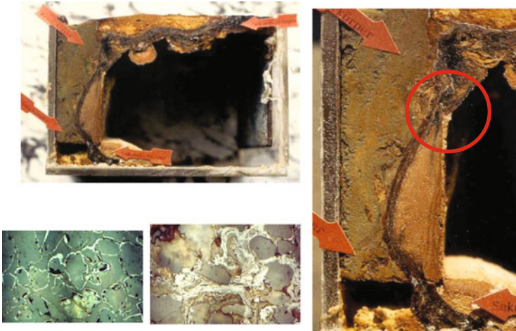
Fig. 8 Laboratory experiment with vertically positioned electrodes, so-called “vein experiment”. (Top left) Full image of the 20 cm × 20 cm × 15 cm test container; (Right) Enlarged section of the symmetrically evolved veinlet; (Bottom left) Ore microscopy analysis Step I: shows quartz grains surrounded by magnetite-like cockade ore; (Center left) Step II: square section of 20 mm: the quartz grains dissolved and banded magnetite deposited instead. It looks like a “hydrothermal ore-vein”. Photographs K.-H. Jacob
