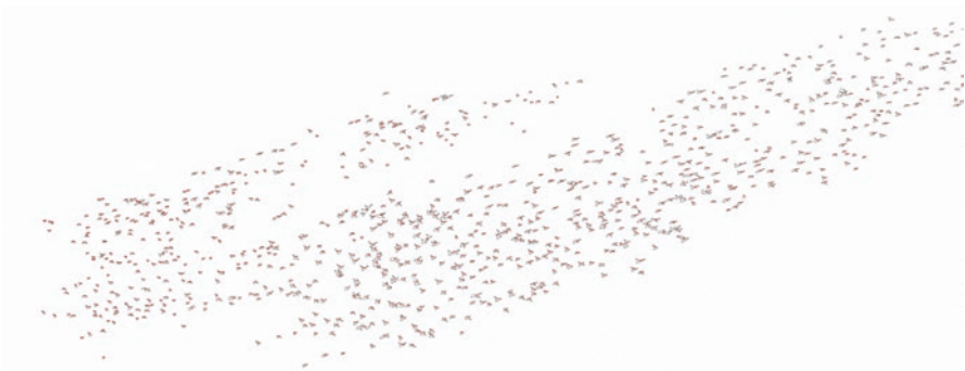
Fig. 12 The drawing generated during the automatic count of the flamingos in flight shows that the counted objects correspond very closely with the distribution of birds in the original image (Fig. 2)
