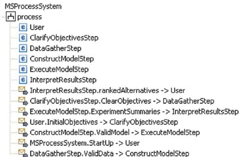
Fig. 3.3 Outline of the MSProcess SES showing coupling
