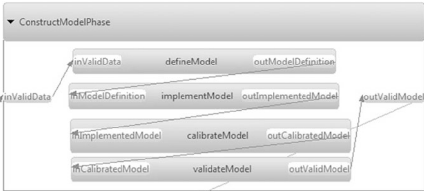
Fig. 3.9 Decomposition of ConstructModels
