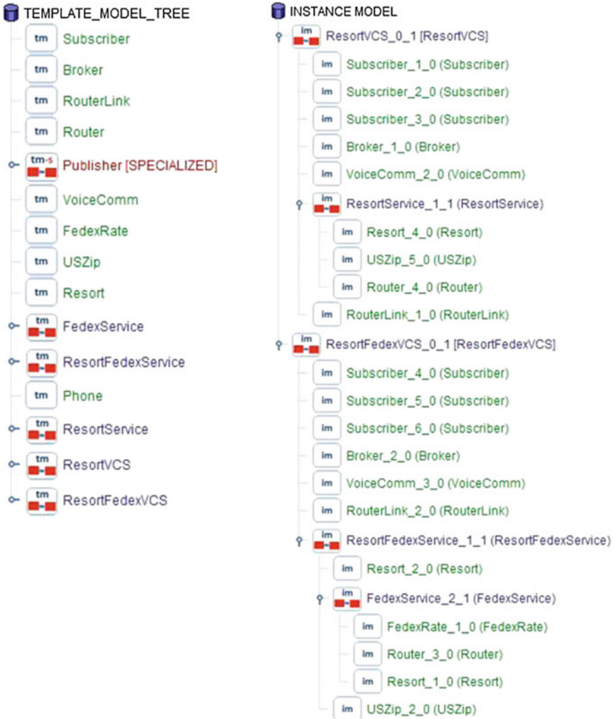
Fig. 16.15 Template and instance models for the instance template models shown in Fig. 16.14
