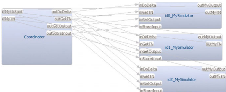
Fig. 9.8 Standard DEVS Protocol with multi-aspect coupling
