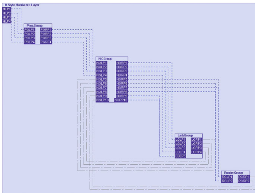
Fig. 16.16 H-Style hardware system model
