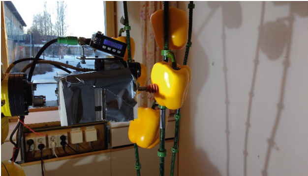
Fig. 5. The pose of each pepper was measured by manually moving the robotic arm in the desired approach direction to the position where the gripper touched the fruit.
