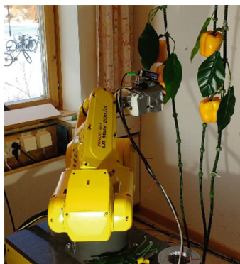
Fig. 1. The experimental setup consisted of a robotic harvester in front of an artificial crop.
