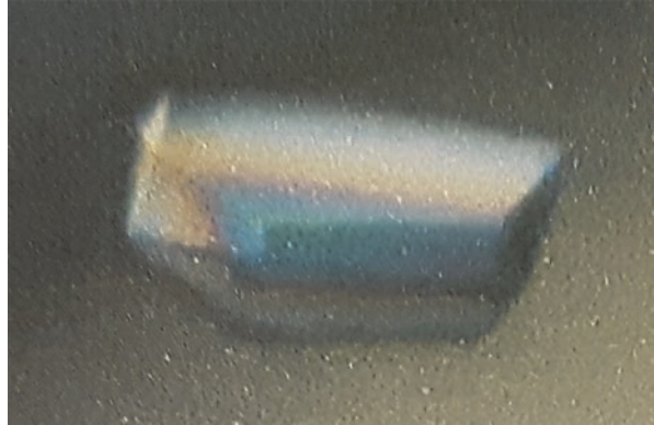
Fig. 2.7 5S RNA crystal grown during IML-2 shuttle mission STS-65 applying the APCF hardware (Förster et al. 2011)
