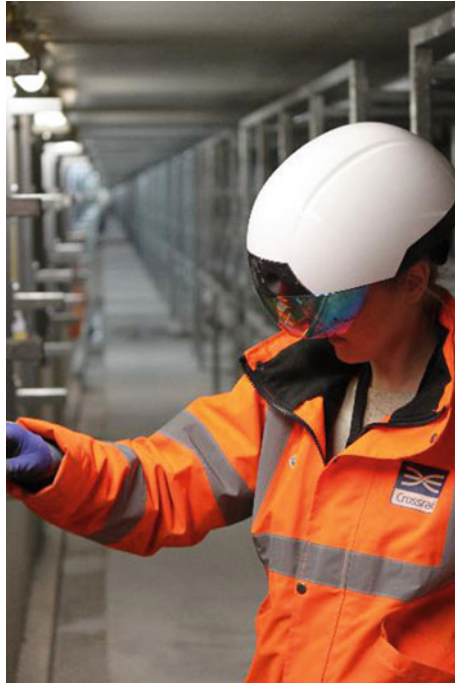
Fig. 4 The In-Site application used at Crossrail’s Liverpool Street station site, by contractor Laing O’Rourke, inspecting assets
