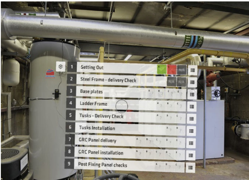
Fig. 5 Point of view from user of the in-site application through the DAQRI smart helmet
