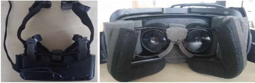
Fig. 2 Oculus Rift DK2 adapted for fNIRS
