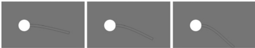
Fig. 6.2 Configuration of the esm-1 benchmark problem and modifications with larger gravity force. Left g_s = -2 , middle g_s = -4 and right g_s = -8
