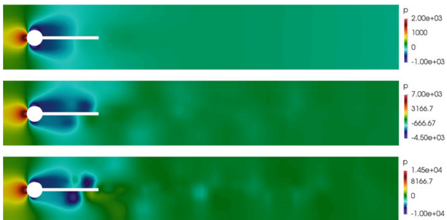
Fig. 11.3 Pressure profile for the flow around a fixed obstacle at different Reynolds numbers. From top to bottom: Re = 100, 200, 300
