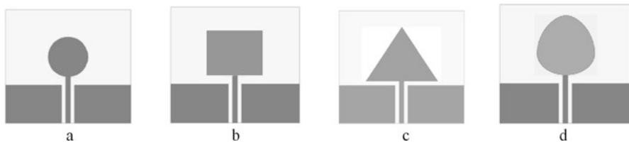
Fig. 1.3 Popular shape of monopole radiators with coplanar waveguide feeding technique, (a) circle, (b) rectangular, (c) triangular, (d) elliptical
